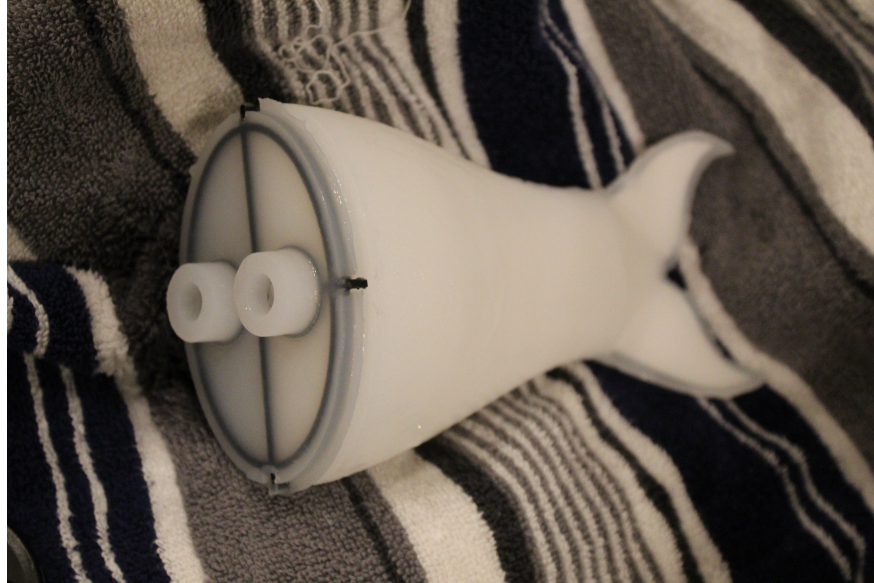
Figure 14: This is what the completed tail assembly should look like for the second tail without the tubing.
