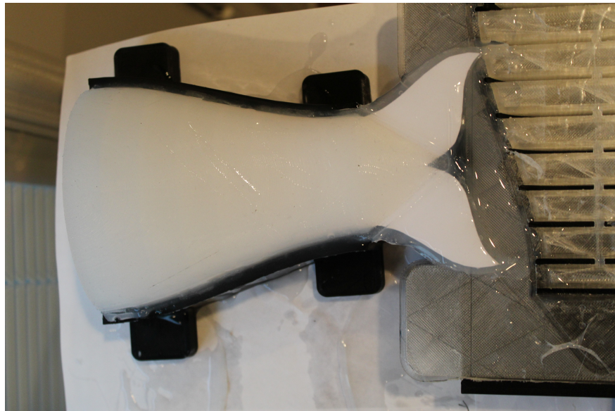
Figure 12: This shows what the setup looks like for the last curing step for the Soft Tail.
