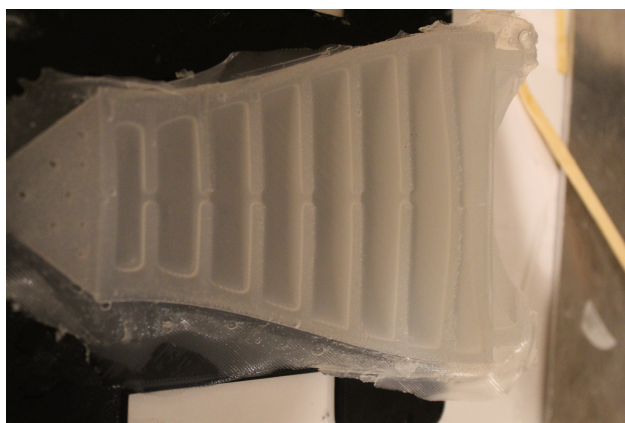
Figure 6: This is a completed Half Tail Piece. Notice that there is a clean channel that connects all of the pockets.
