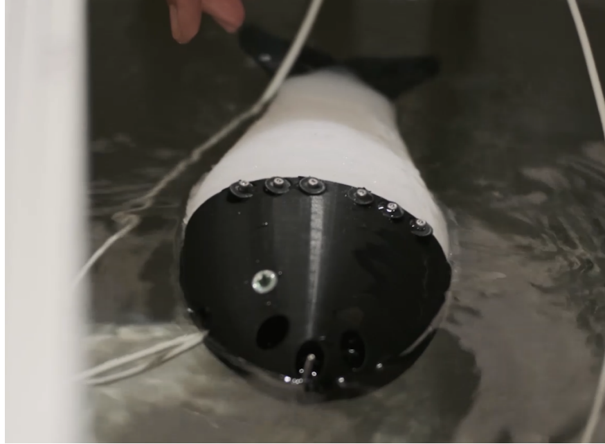
Figure 17: The first tail assembly floats in the water when its chambers are filled with air.
