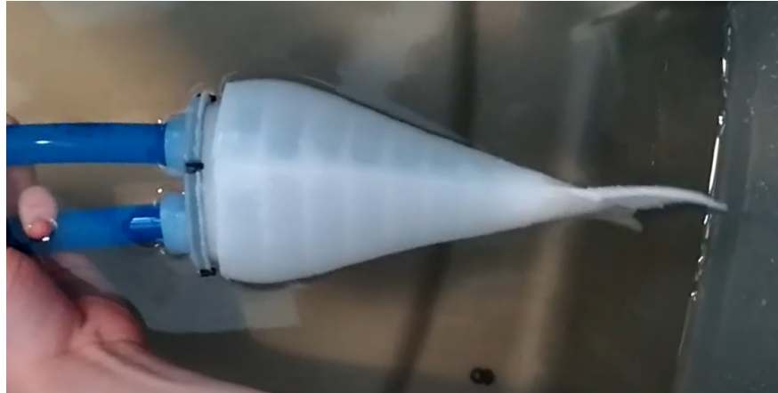
Figure 19: The second tail successfully moves back and forth underwater. However, the second tail does not curve nearly as much as the first tail.
